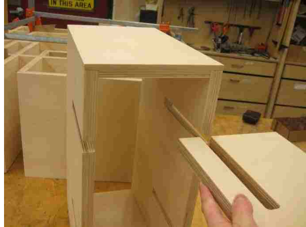
Fig. 9.5 Interlocking slot detail and assembly
